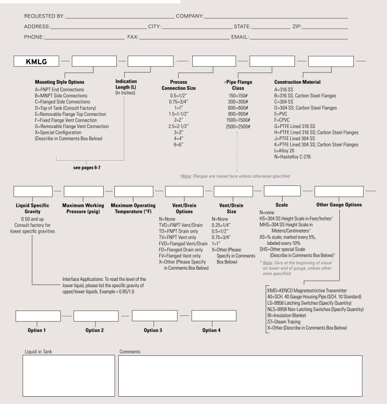
Example: [KMLG-C-36-2-150-A-0.71-175-100-TVD-0.5-HS-LS(2)] is a Magna-Site with flanged side connections, 36" indication length (L), 2" 150 lb. R.F. flanged process connections, 316 stainless steel construction, float specific gravity of 0.71, a maximum working pressure of 175 psig at 100°F, 1/2" FNPT vent/drain, a 304 stainless steel height scale in feet/inches, and (2) 9958 latching switches.
