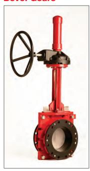
Bevel gears are recommended for high-pressure service or larger diameter valves. Suggested on all DX Valves over 6" in diameter and above 75 psi working pressure.
