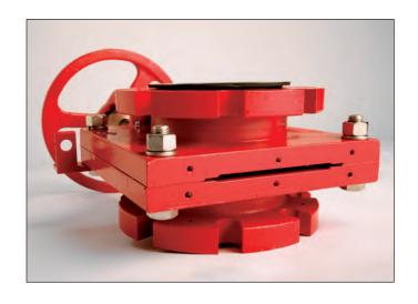
Each time the DX Valve strokes, it discharges a small amount of slurry, which keeps the gate path and seat area clear of entrapped particulates. Unlike traditional knife gate valves, the DX Valve prevents slurry build-up in the seat area, which might otherwise prohibit the valve's ability to close. Both the slurry sleeves and gate are field replaceable.
