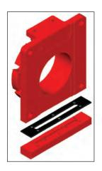
The new DX Valve has an optional cleanout area at the base of the body for splash containment. At the bottom of the valve is a removable drain plate. The clean-out area should be considered as a way to eliminate the need for an external splash guard, or can be utilized as a flush or purge connection.
