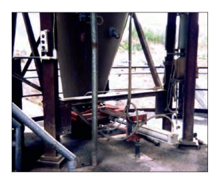
A portable hydraulic power unit can be specified to actuate the DX Valve. A transportable unit is especially convenient for actuating valves in out-of-reach or inconvenient locations, such as tailing lines. Also common is the use of one portable hydraulic unit to actuate multiple valves in close proximity, as found at a cyclone separator.
