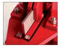
A wiper blade mounted on the top of the valve prevents the gate lubricant and process from leaking through the top. The DX Valve design eliminates the need for traditional packing. This wiper blade also prevents external grit from entering the valve body.
