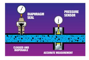
The Series 40W pressure sensor isolates and protects instrumentation. The full-port design eliminates clogging, ensuring accurate pressure measurement under the most difficult conditions. The elastomer sleeve senses pressure 360 degrees around the inner circumference of the unit, overcoming problems like plugging and fouling of traditional diaphragm seals.
