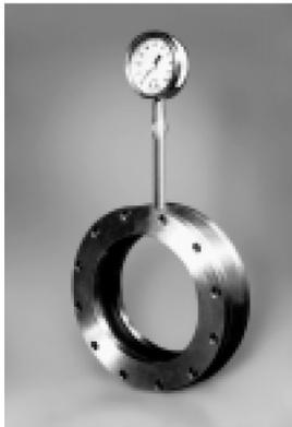
Red Valve's Series 48R Pressure Sensor protects and isolates instrumentation, eliminating plugging and fouling that can occur in slurry and hard-to-gauge liquid applications. The economical Series 48R is designed to fit inside the bolt pattern of the pipe flanges, allowing for ease of installation and reducing the size of the unit. Series 48R sensors are designed to fit Class 150 and 300 flange drilling, DIN, or BS NP10 piping systems.
