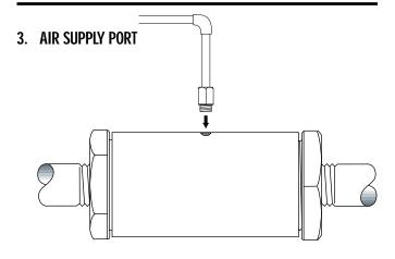
Air supply is connected to the 1/4" NPT port. This port is normally plugged on the 2633, but can be used as a drain or piped as a flush port. Use the chart below to determine the correct air pressure needed to close the 2600.
