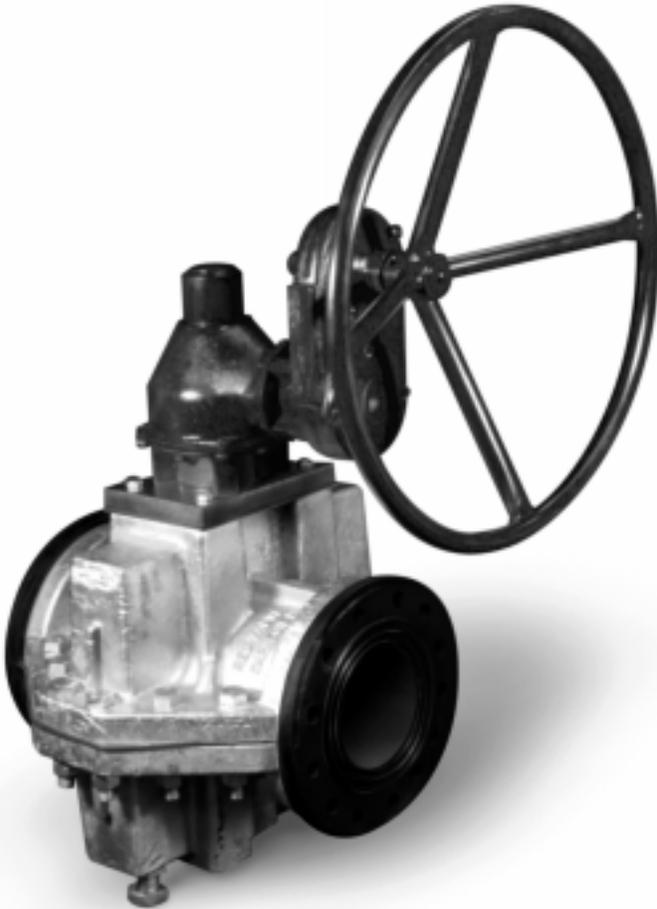
The Red Valve Series 9000 manually actuated Pinch Valve is a bi-directional valve designed for tough slurry applications. The elastomer sleeve closes on entrapped solids in the line. The flexing action of the sleeve breaks up any sediment or build-up in the valve, which makes the Series 9000 a reliable, low maintenance valve.
