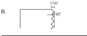
B. It is recommended that the mating flange be serrated to "grip" the rubber flange. The serrations should be cut 1/16" deep, with a 90 degree tool point. The pitch should be 8 (eight) cuts per inch.
