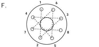
F. Torque all the flange bolts in a star pattern, first to 50% of tabulated valves, then retorque to 100% of tabulated valves. If greater torque is required, continue retorquing in increments of 50% of tabulated valves. Use of high quality anti-seize compound on all bolt threads is recommended.
