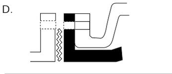
D. When installing a pinch valve to a rubber, PVC, or any "slick" mating flange, we recommend that you install a metal serrated gasket between the two flanges to assist in the seal.
