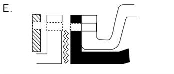
E. When bolting a pinch valve to a PVC or synthetic mating flange, use a split back-up retaining ring, since the mating flange will yield prior to generating enough force on the flange faces for a proper seal.
