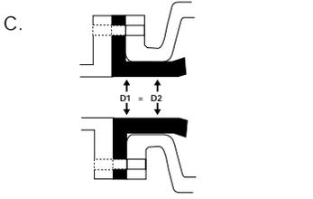
C. Mating flange ID must match the pinch valve sleeve ID.
