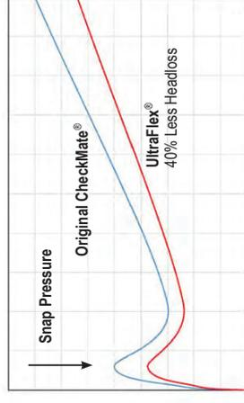
The new CheckMate UltraFlex® Valve boasts a 40% lower snap pressure requirement to open or unseat the valve, without compromising the valve's ability to seal. This greatly improves capacity in pipelines and the rapid drainage of upstream flow through the valve. With its patented "Arc Notch" design, the CheckMate UltraFlex® Inline Check Valve boasts a significantly improved flow efficiency, due to reduced head pressure levels required to "snap" open the valve.
