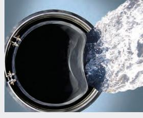
When upstream head reaches 50-75% of pipe diameter (for example, 9" head in a 12" valve), the UltraFlex® bill "snaps" open into a concave shape, allowing substantially more flow with the same amount of head. The valve will progressively open with increased head and flow. Picture shows moment when the valve "snaps" open.
