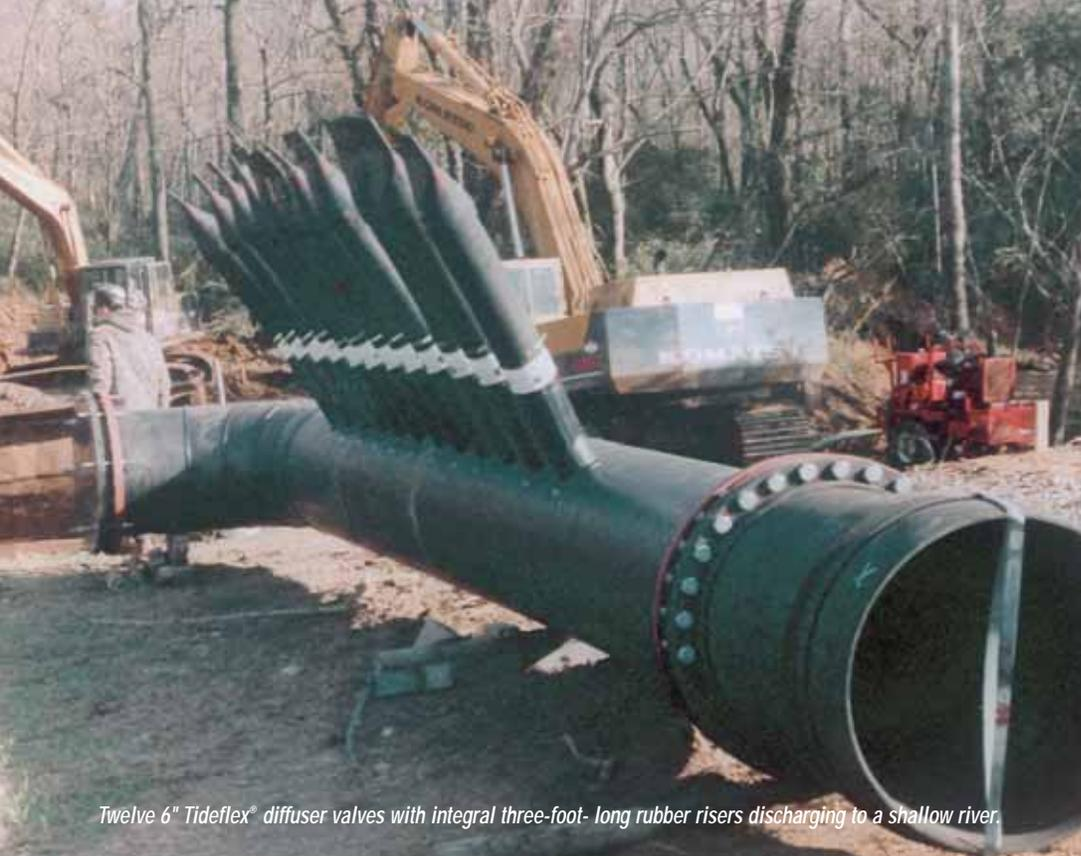
Twelve 6" Tideflex® diffuser valves with integral three-foot- long rubber risers discharging to a shallow river.
