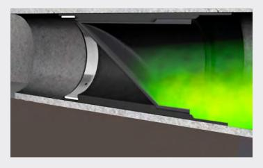
CheckMate® Inline Check Valves use state-of-the-art elastomers and fabric technology with no metal hinges, rivets, fasteners or moving parts. The valve's unibody construction is ideally suited for CSO and diversion chamber applications, installed at the upstream or downstream side of a diversion chamber. When used in interceptor and manhole installations, they prevent unwanted backflow and odors from damaging the community.
