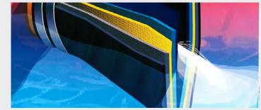
What sets Red Valve products apart from traditional valves is leading-edge elastomer technology. In addition to providing a superior flow pattern, the rubber sleeve provides unsurpassed abrasion and corrosion resistance, closing drop-tight around entrapped solids.
