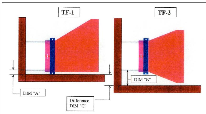
Another major benefit of the TF-1 is the valve allows the invert of the pipe to be lower since it does not require as much bottom clearance. This results in a greater hydraulic capacity of the outfall because the slope of the pipe is increased, which maximizes the amount of driving head available to pass flow.
